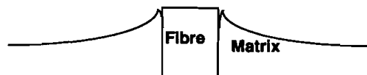
Figure 1. Exaggerated schematic view of the interfacial crack due to the free edge effect in a single fibre composite after being processed
