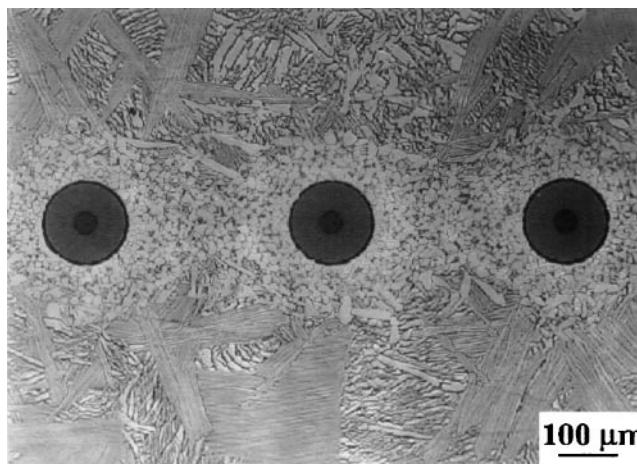
FIG. 4. Optical micrograph showing the matrix microstructure around three fibers in a Ti-6Al-4V/SiC single-ply composite which was consolidated in the supra-transus region.
