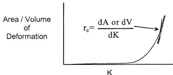
Figure 8: Criteria for failure: critical rate of deformation growth with respect to change in stress intensity factor
