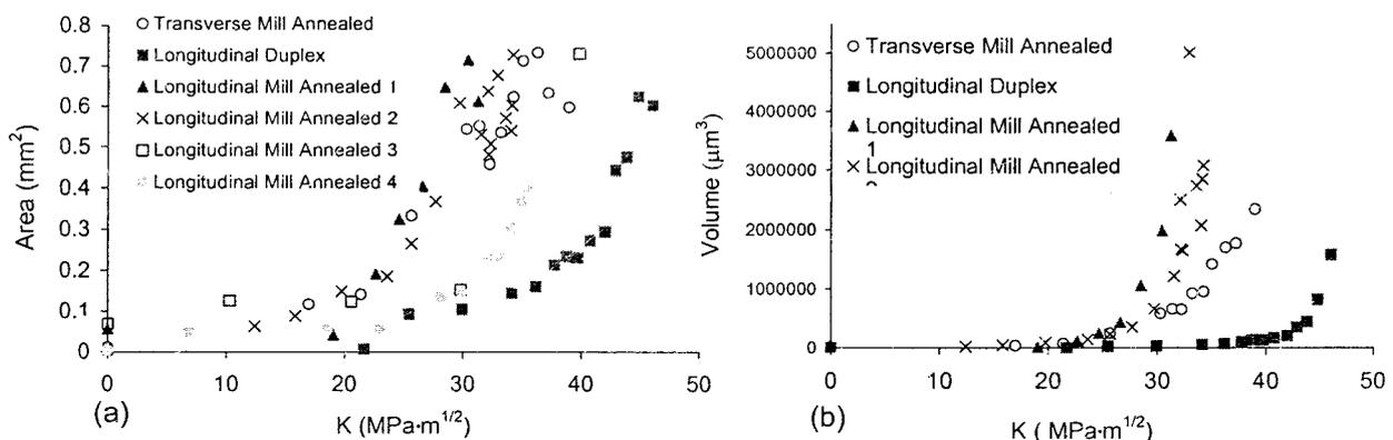
Figure 3: Deformation and stress factor relationship for Ti-6Al-4V for (a) area and (b) volume
