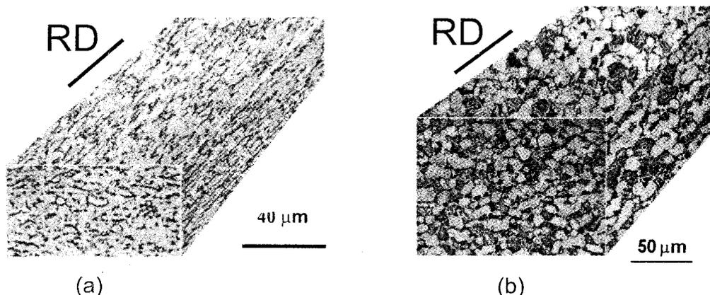
Figure 1: Microstructure of Ti-6Al-4V specimens (a) mill annealed sheet and (b) duplex microstructure forged plate
