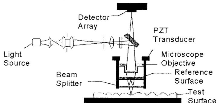
Figure 2: Schematic of White Light Interference Profilometer
