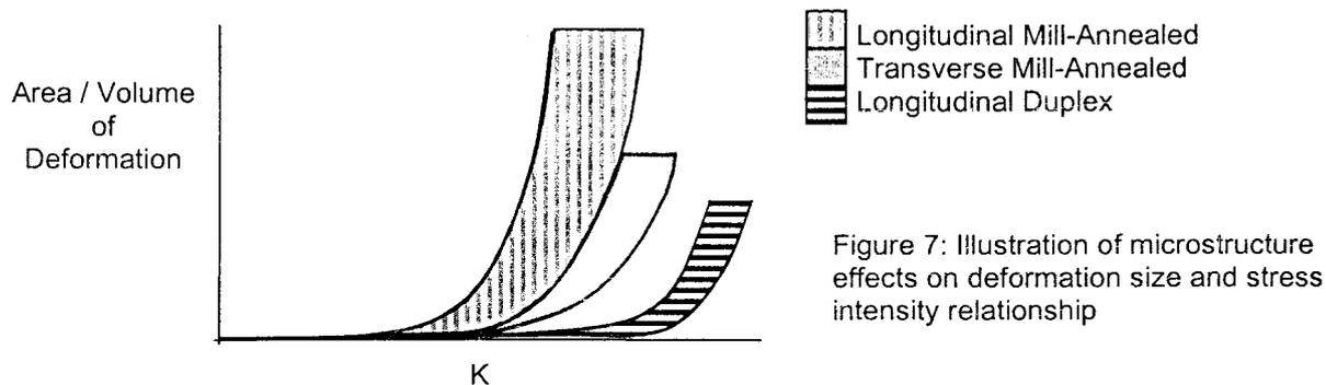
Figure 7: Illustration of microstructure effects on deformation size and stress intensity relationship
