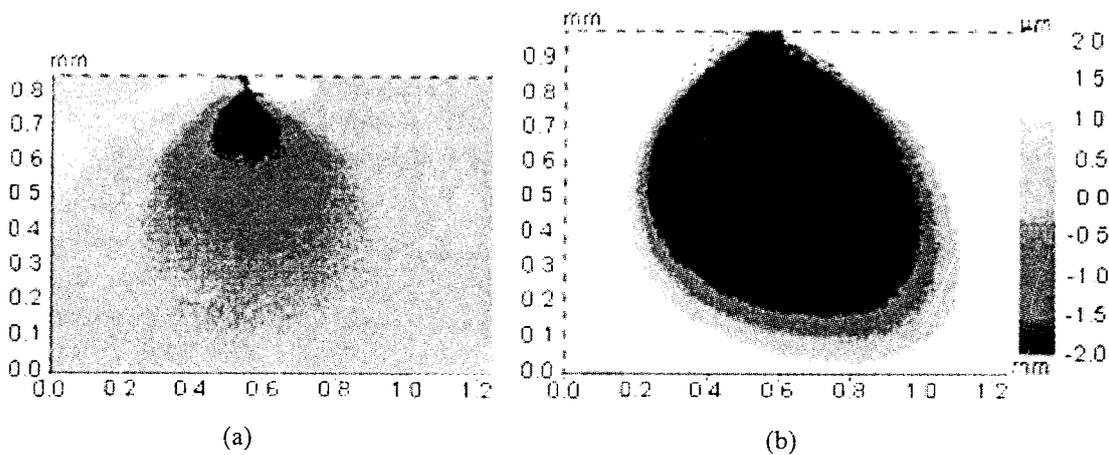
Figure 5: Deformation zones under loads of (a) 2500 N and (b) 3500 N (directly before failure)
