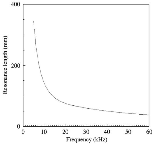
Figure 4. Dependence of sample resonance length on ultrasonic frequency for Ti-6 Al-4V.
