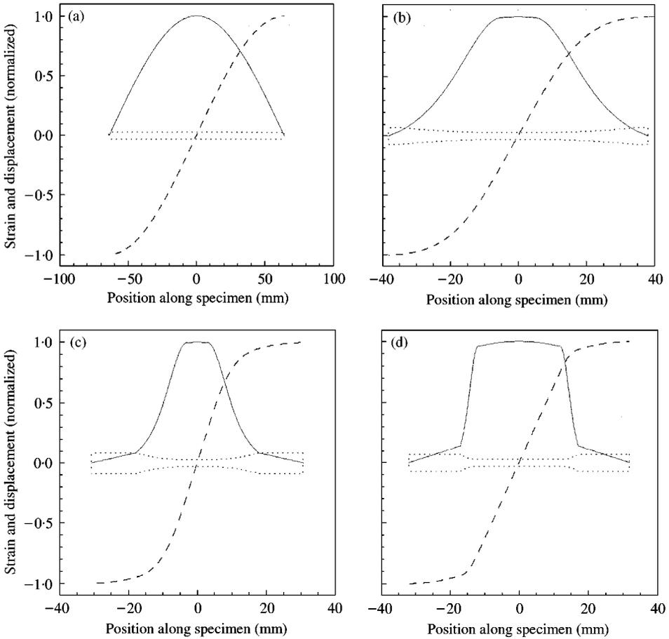
Figure 2. (a) Strain (—) and displacement (---) distribution for cylindrical Ti-6 Al-4V specimen. The specimen geometry is shown by (···) line; (b)-(d) strain (—) and displacement (---) distribution for dog-bone Ti-6 Al-4 V specimen (geometry shown in Table 1). The specimen geometry is shown by ··· line.
