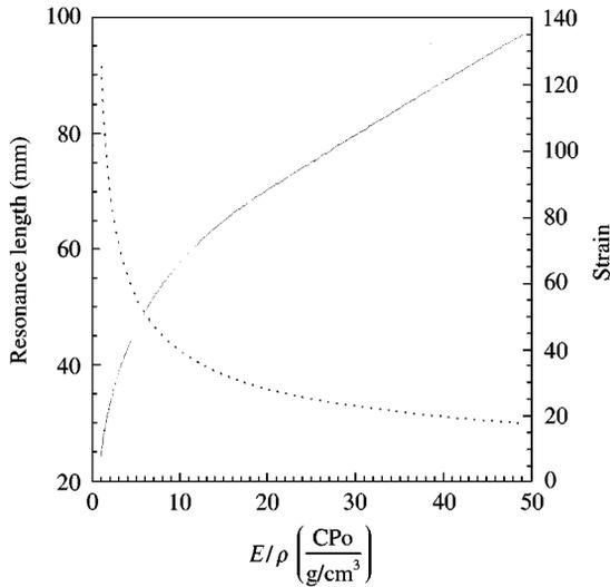
Figure 3. Maximum strain (····) and resonance length (—) as a function of material properties.
