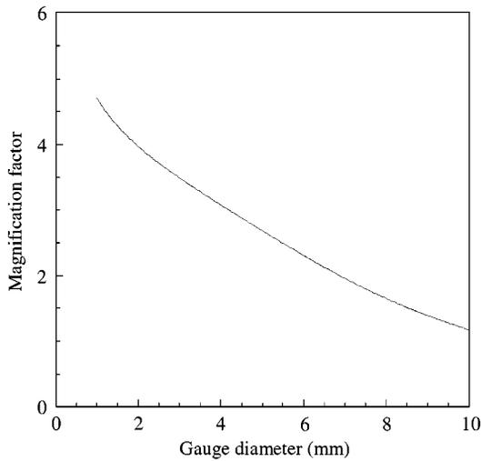
Figure 5. Magnification versus diameter at the center of the specimen (gage diameter).
