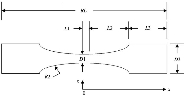
Figure 1. Longitudinal section of dog-bone-shaped specimen:  $L1$ , gage length;  $D1$ , gage diameter;  $L2$ , transition length;  $R2$ , radius of curvature;  $L3$ , end length,  $D3$ , end diameter;  $RL$ , resonance length. The center of the specimen corresponds to  $(x = 0, z = 0)$ .
