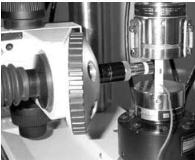
FIGURE 4 Alumina matrix tested in axial compression with simultaneous fluorescence measurements
