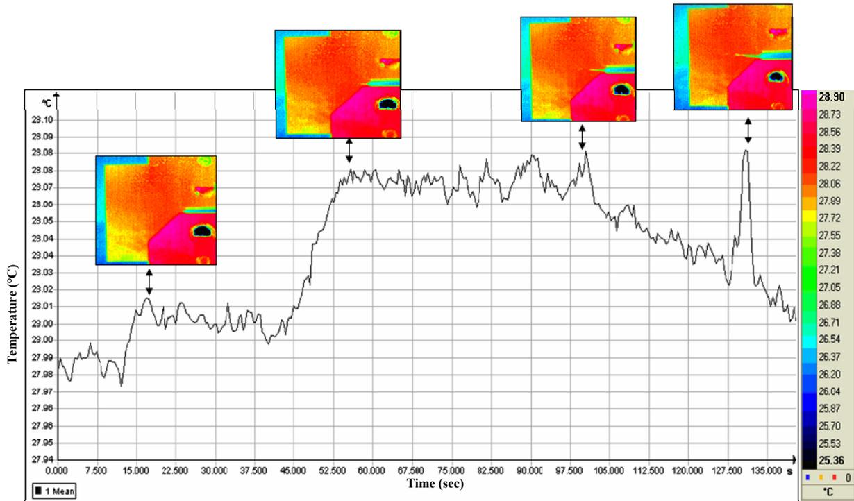
**Fig.5d** Thermographic monitoring of Al/SiC<sub>p</sub> HT1 composite CT specimen showing the different stages of crack growth up to the sample's final fracture.
