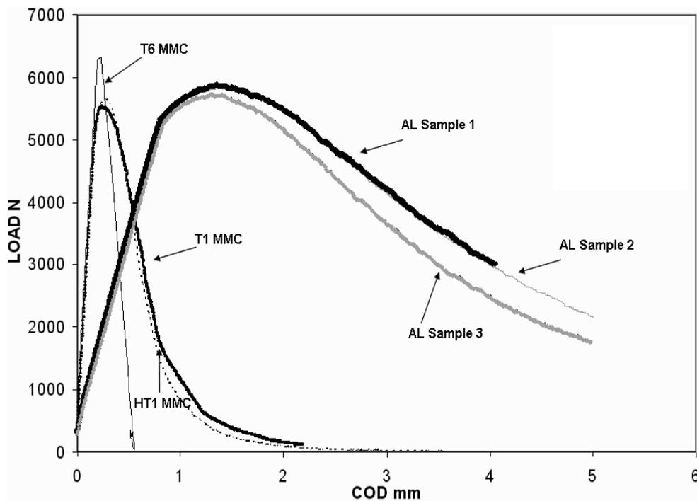
**Fig.3** Load – Displacement curves for Al/SiC<sub>p</sub> composites subjected to T1, T6 and HT-1 heat treatment conditions and three unreinforced aluminium alloy samples.
