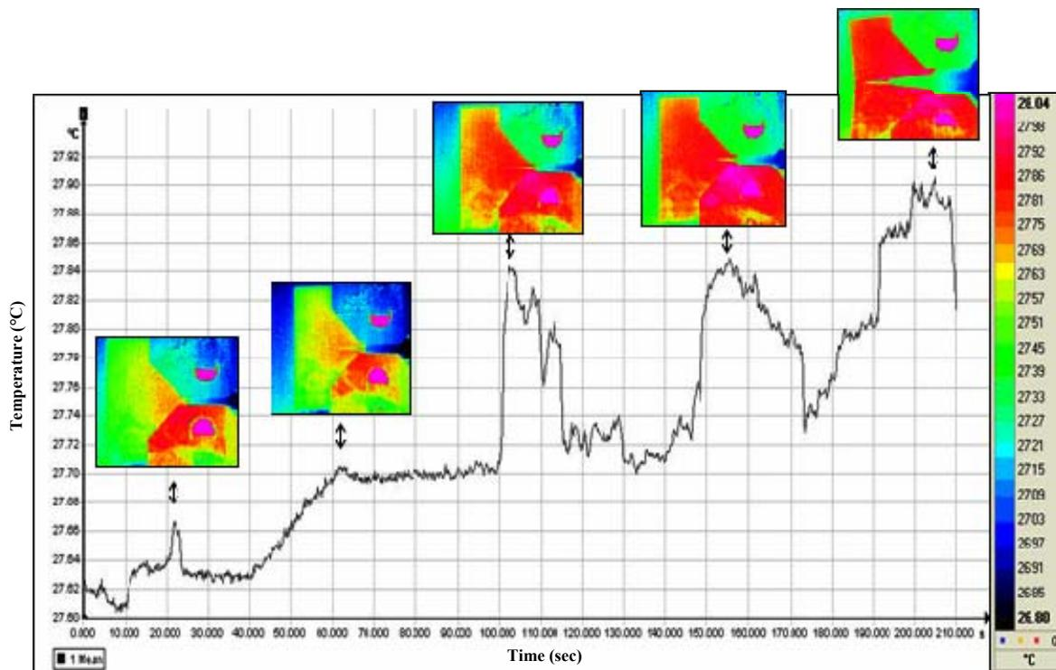
Fig.5c Thermographic monitoring of Al/SiCp T6 composite CT specimen showing the different stages of crack growth up to the sample's final fracture.
