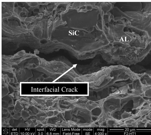
**Fig.6b** HT-1 heat treatment condition: cracking through interface.
