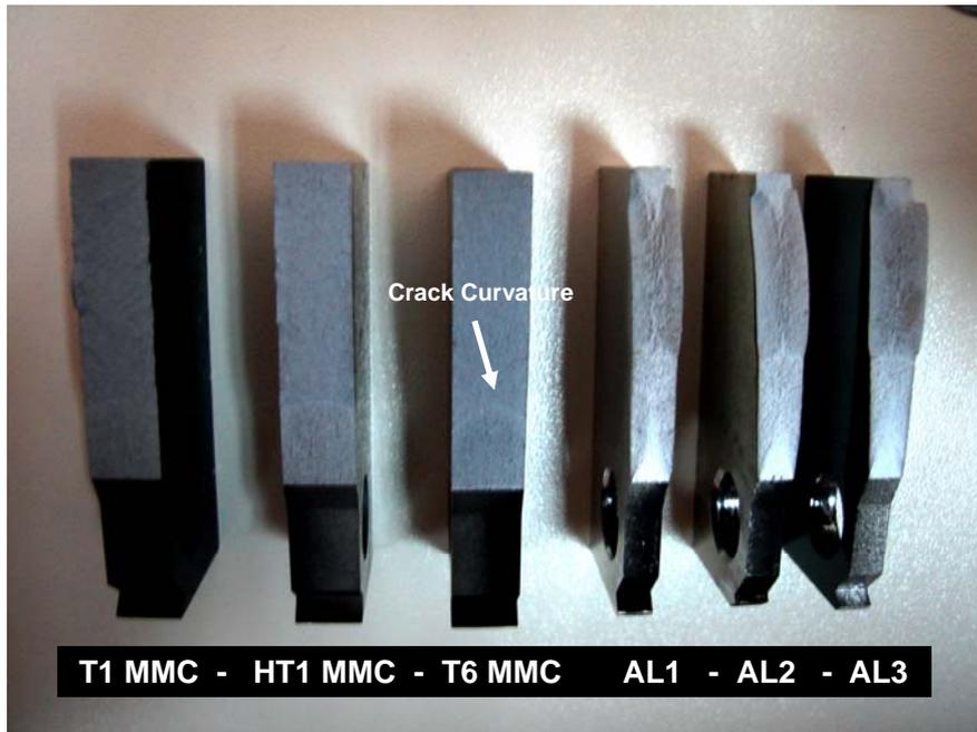
**Fig.4** Variation in crack curvature with specimen thickness.
