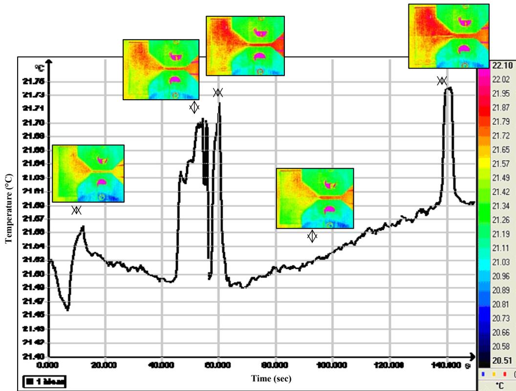
Fig.5b Thermographic monitoring of Aluminium 2xxx CT sample showing the different stages of crack growth up to the specimen's final fracture.
