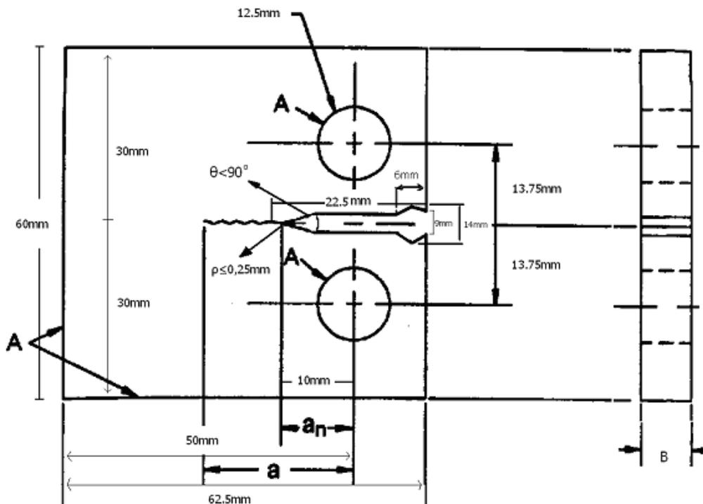
**Fig.2** Fracture Toughness CT specimen geometry according to ASTM E399 standard.
