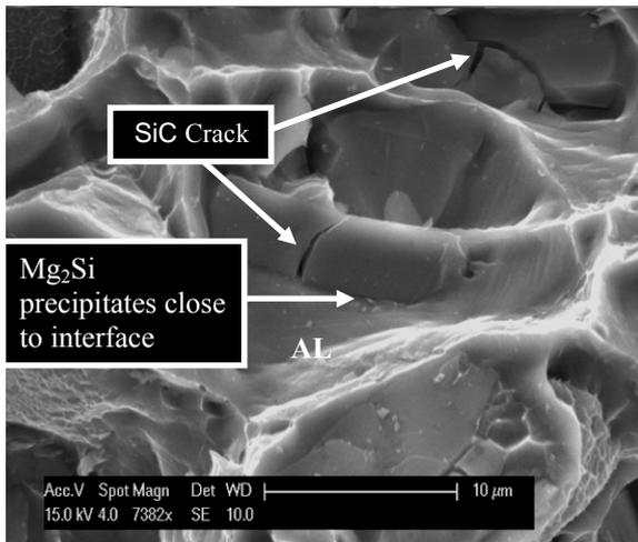
**Fig.6a** T6 heat treatment condition: SiC particles cracked but not debonded.
