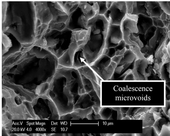
**Fig.6c** As received condition: Presence of coalescence microvoids indicating ductile behaviour.
