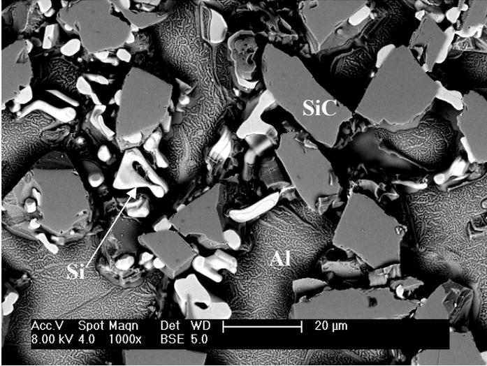
**Fig.1** SEM image showing an aluminium – silicon – magnesium alloy matrix, A359, reinforced with 31 wt. % silicon carbide particles.
