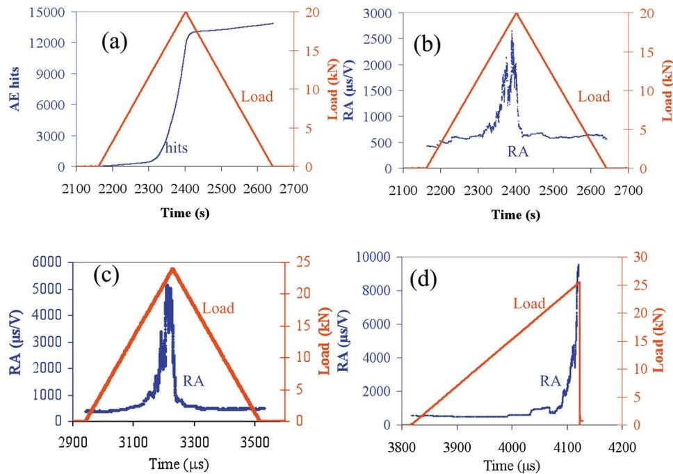
Fig. 1. (Color online) (a) Load history and AE cumulative hits for step 5, load history and RA value for step 5 (b), step 6 (c), step 7(d).
