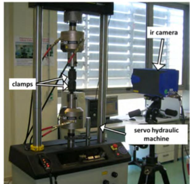
Fig. 2. Photograph of the sensors on the specimen. Fig. 3. Photograph of the experimental setup.
