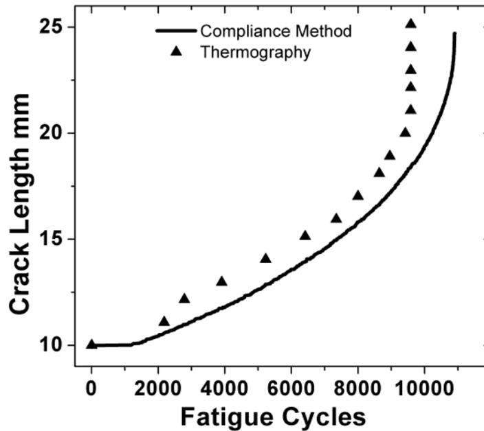
Fig. 10. Crack length vs. fatigue cycles determined by the compliance method and thermography.
