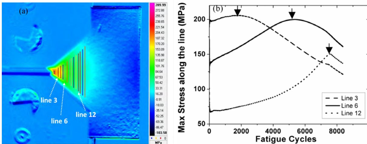
Fig. 9. (a) thermograph of 3 plotted reference lines s, (b) Diagram of max stress along 3 typical reference lines vs. fatigue cycle.
