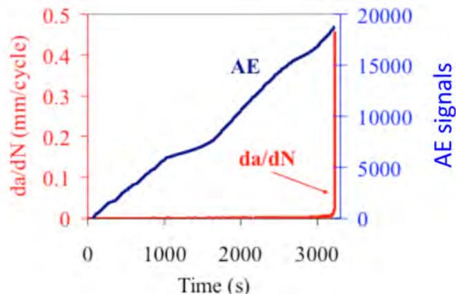
Fig. 4. Time history of CPR (or  $da/dN$ ) and cumulative AE.
