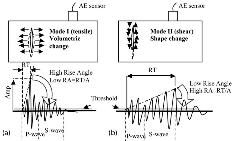
Fig. 1. Cracking modes and corresponding AE signals.
