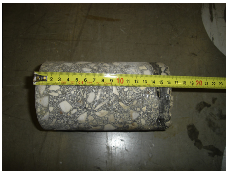
Fig. 10. Concrete core, cut off after the grout injections, with visible grout attachment on the bottom side.
