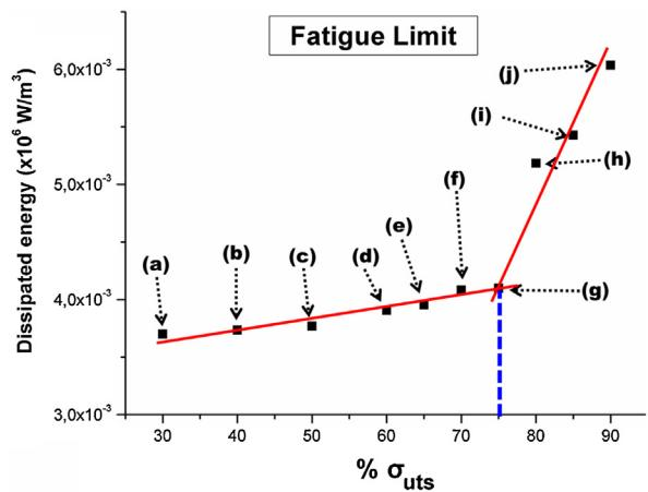
Fig. 3. Dissipated energy vs % $\sigma_{\text{uts}}$  (Al 1050 H16).
