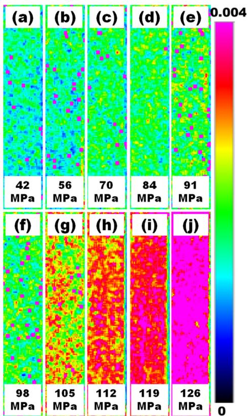
Fig. 4. Thermographs for Al 1050 H16 specimens.
