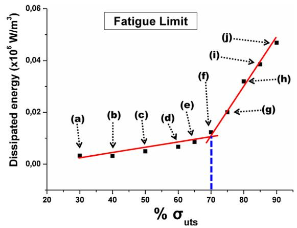
Fig. 6. Dissipated energy vs % $\sigma_{uts}$  (SiC/BMAS).
