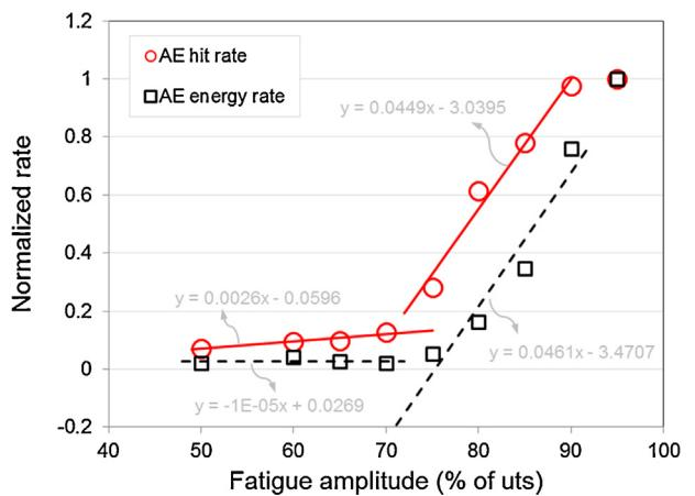
Fig. 9. Rate of increase of accumulated hits and energy.
