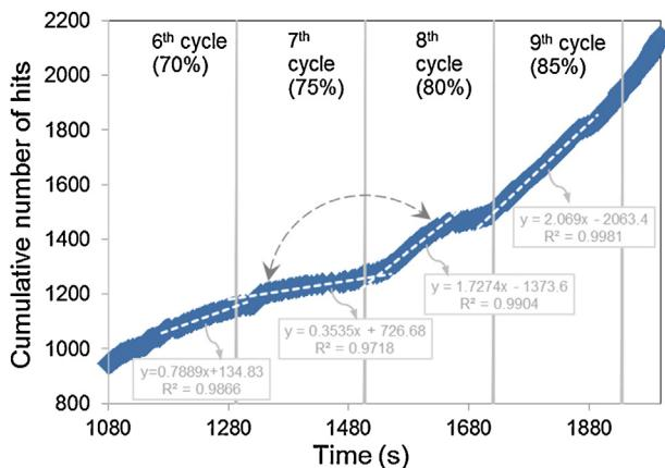
Fig. 5. Cumulative AE activity for different loading stages of aluminum specimen.
