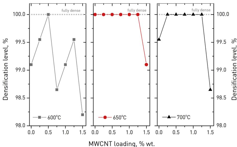
Fig. 3. Densification levels of MWCNT/borosilicate glass materials with varying nanotube concentrations as a function of sintering temperature (600, 650 and 700 °C). The y-axis values are obtained by normalization of CNT/ceramic densities measured via the Archimedes method, to 2.22 g/cm<sup>3</sup>, the property value achieved for fully dense pure borosilicate glass samples (0% MWCNT loading).
