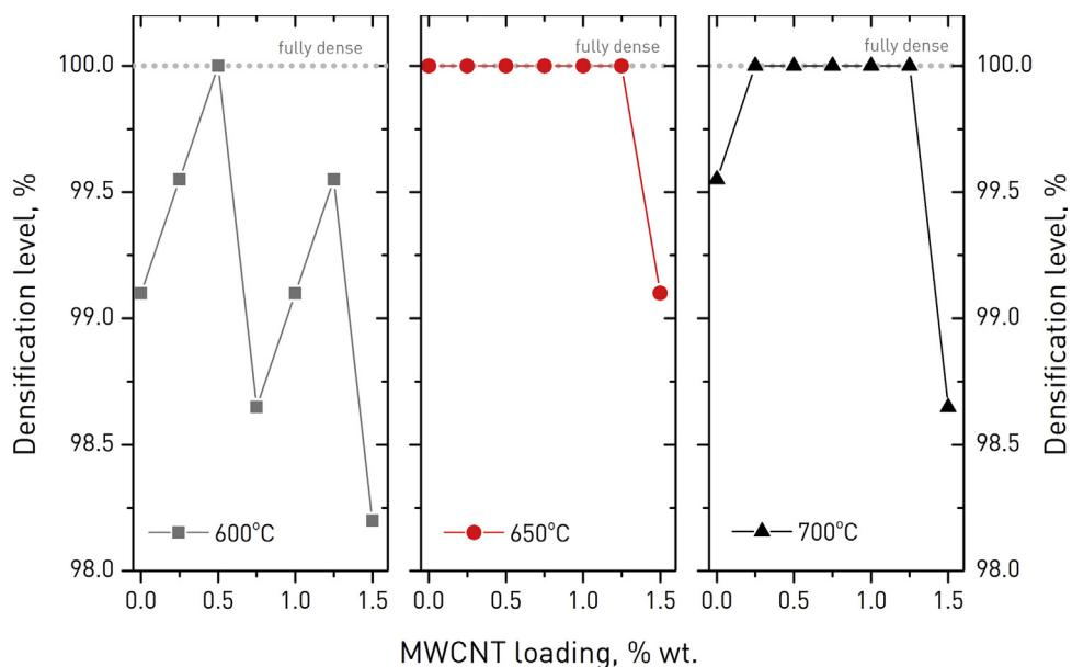
Fig. 3. Densification levels of MWCNT/borosilicate glass materials with varying nanotube concentrations as a function of sintering temperature (600, 650 and 700 °C). The y-axis values are obtained by normalization of CNT/ceramic densities measured via the Archimedes method, to 2.22 g/cm<sup>3</sup>, the property value achieved for fully dense pure borosilicate glass samples (0% MWCNT loading).
