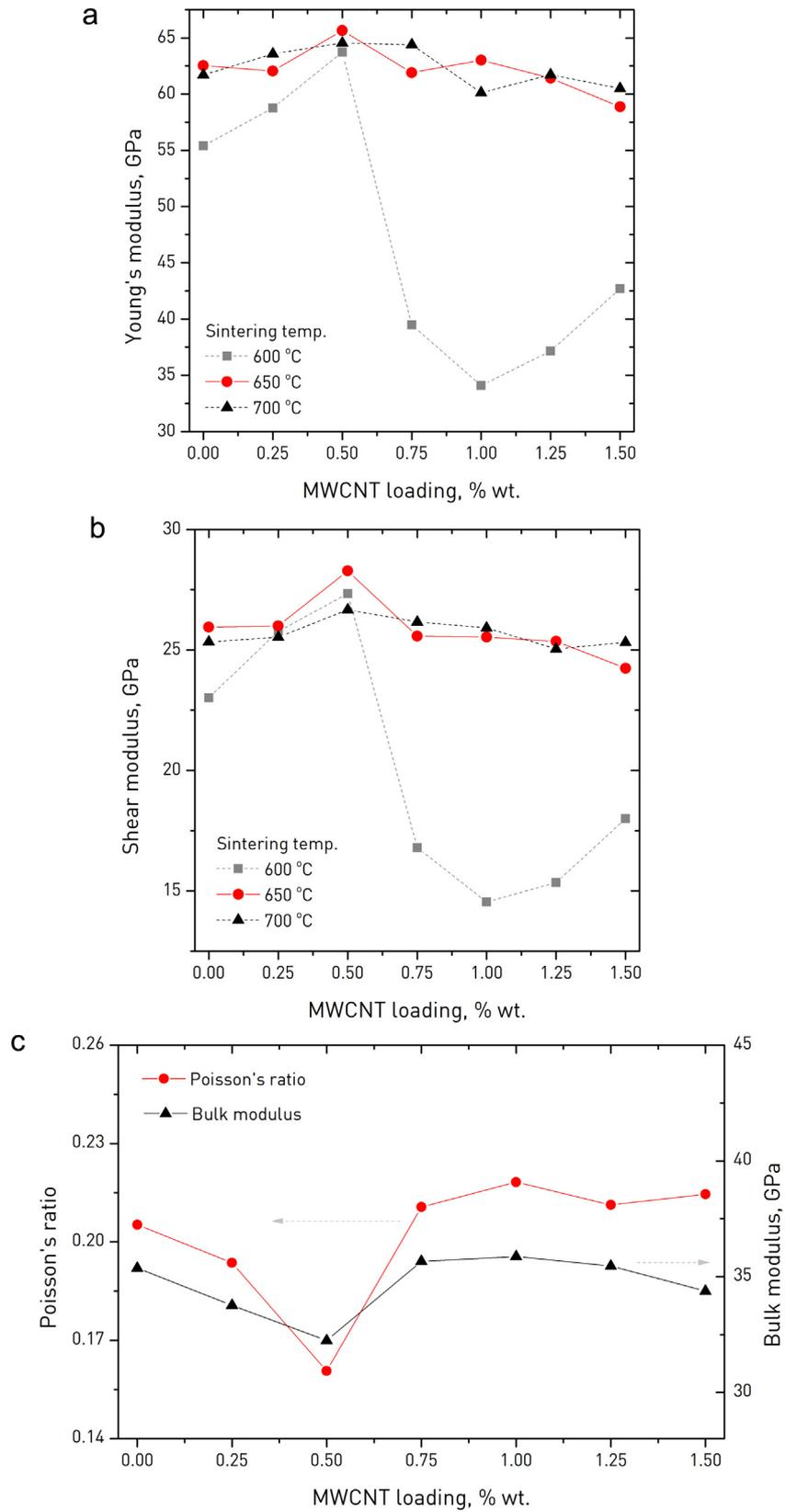
Fig. 4. Dynamic mechanical properties of MWCNT/borosilicate glass versus tube loading: (a) Young's modulus, (b) shear modulus for samples sintered at 600, 650 and 700 °C and (c) Poisson's ratio (red solid cycle symbols) and bulk modulus (black solid triangle symbols) of fully dense samples sintered at 650 °C. (For interpretation of the references to color in this figure legend, the reader is referred to the web version of this article.)
