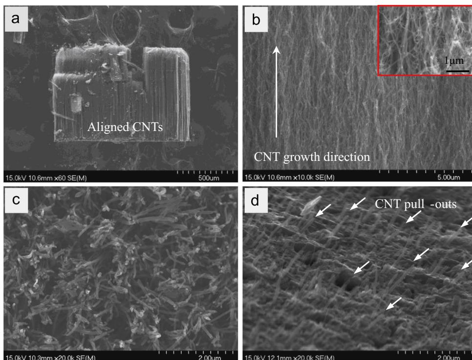
Fig. 1. SEM micrographs showing (a) the pristine VACNT forest piece, (b) vertical CNT alignment in the forest, (c) cross-section of forest showing open porosity and (d) numerous MWCNT pull-out tips in the fractured section of VACNTs/SiC composites.
