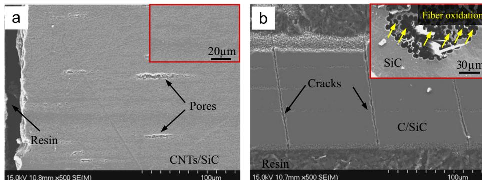
Fig. 3. SEM micrographs of the polished surface of (a) VACNT/SiC composite and (b) plain C/SiC composites prior to oxidation tests. Insets show higher magnifications of the surfaces of polished VACNTs/SiC and fiber oxidation through the cracked SiC matrix of C/SiC.
