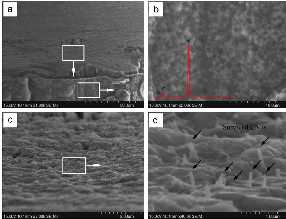
Fig. 4. SEM micrographs showing the fractured VACNT/SiC composites after oxidation: (a) the fracture section of the VACNT/SiC, (b) the surface of composite, where the SiC matrix was oxidized to viscous state silica, (c) a high magnification of the white rectangle in (a), in which plenty of CNT pull-outs were found, and (d) a high magnification of the white rectangle in (c), where the CNT pull-outs were clearly observed without apparent oxidation (black arrow).
