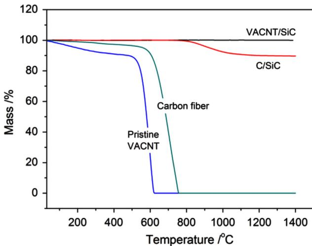
Fig. 2. Thermogravimetric curves of pristine VACNT forests, carbon fibers, plain C/SiC composites and VACNT/SiC composites, in air.
