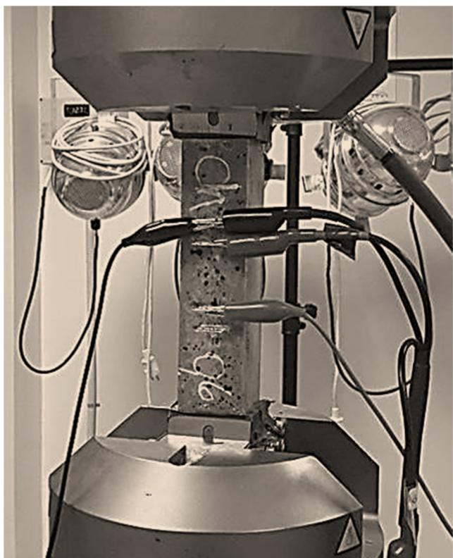
**Fig. 5.** Nano-modified mortar undergoing cycling loading with simultaneous piezoresistivity measurement.
