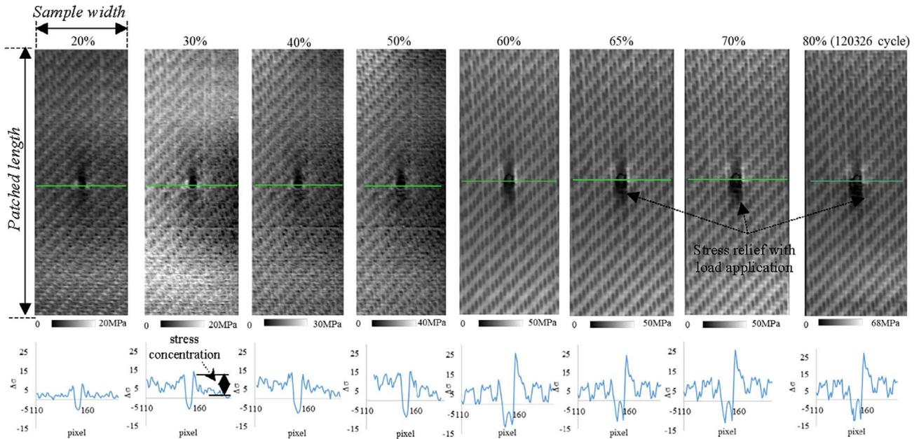
Fig. 7. Progress of delamination/separation/detachment of patch from the substrate during fatigue loading from 20 to 80% of  $\sigma_{uts}$ ; respective normalised amplitude versus distance (pixels) graphs.
