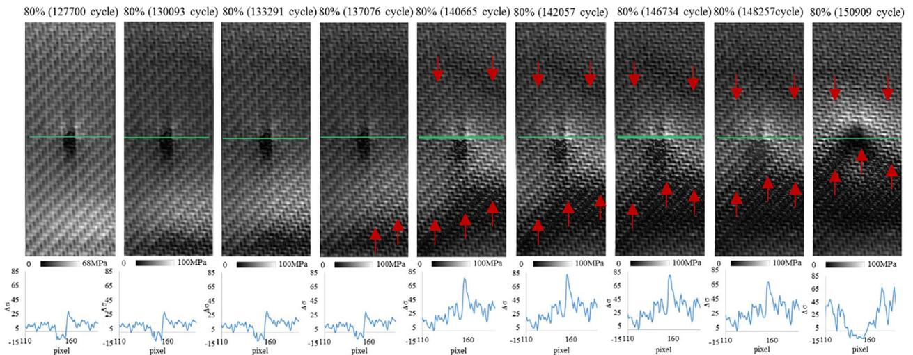
Fig. 8. Progress of delamination/separation/detachment of patch from the substrate during fatigue loading at 80% of  $\sigma_{uts}$  from cycle 127,700 cycle until rupture; respective normalised amplitude versus distance (pixels) graphs.
