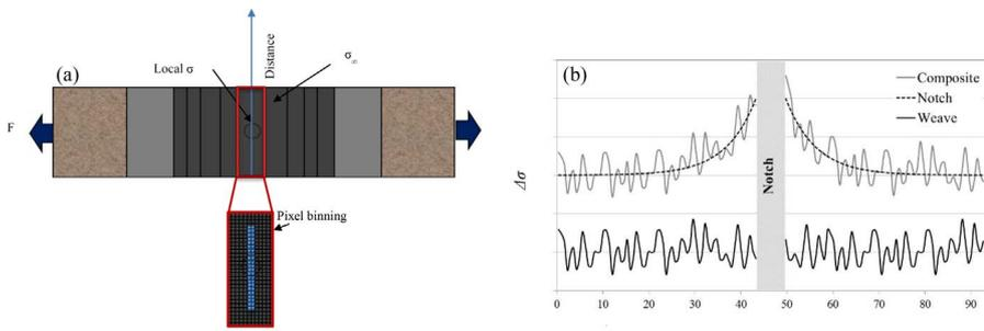
Fig. 6.  $\Delta\sigma_{local}/\Delta\sigma_{\infty}$  ( $=\Delta\sigma$ ) vs. distance: (a) location of measurements, (b) components of the composite graph: weaving pattern and notch induced  $\Delta\sigma$ .
