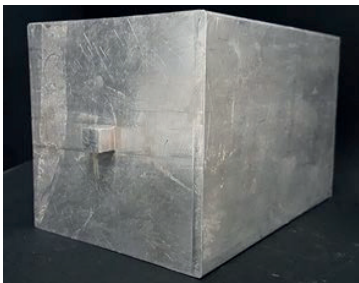
Figure 6. Aluminum waveguide. At the center of the front face of the waveguide appears a small cube of dimensions 10 \times 10 \times 10 \text{ mm}^3 .
