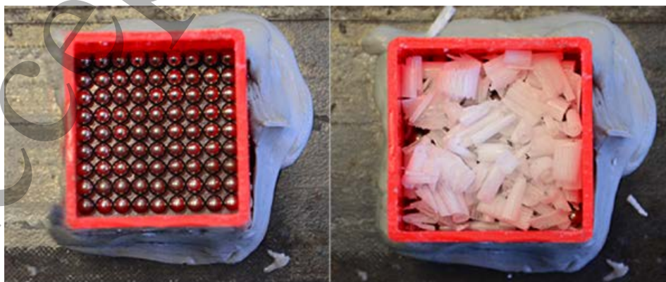
Figure 1. PnC assembly. The white material on the right is the paraffin used.
