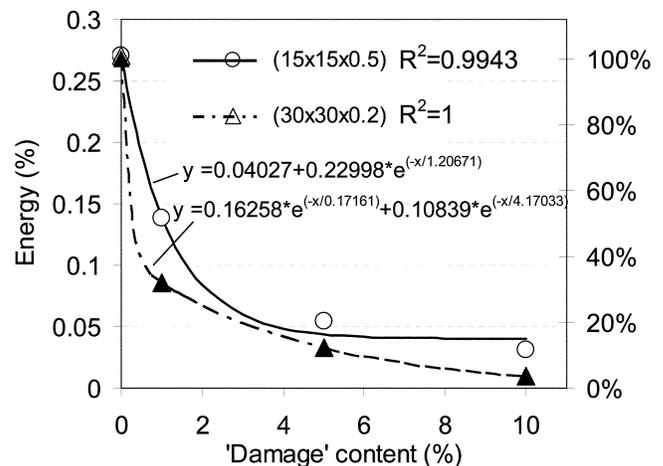
Fig. 4—Waveform energy versus inclusion content for different inclusion size.
