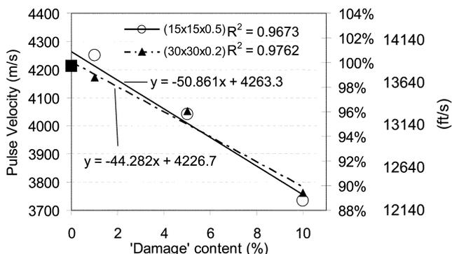
Fig. 2—Pulse velocity versus inclusion content (square symbol stands for plain mortar).
