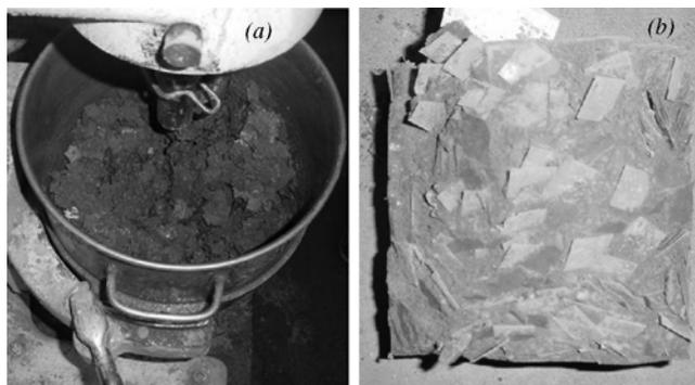
Fig. 1—(a) Mixing of plastic inclusions with fresh mortar; and (b) distribution of inclusions in pilot specimen.
