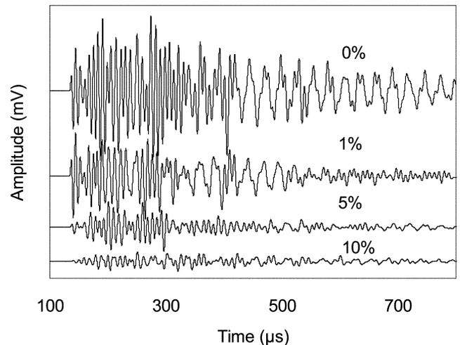
Fig. 3—Waveforms from mortar with different content of inclusions.
