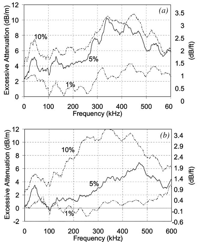
Fig. 8—Attenuation coefficient versus excitation frequency for different inclusion content and inclusion sizes: (a) 30 x 30 x 0.2 mm (1.18 x 1.18 x 0.007874 in.); and (b) 15 x 15 x 0.5 mm (0.59 x 0.59 x 0.02 in.).
