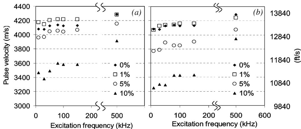
Fig. 6—Pulse velocity versus excitation frequency for different inclusion content and inclusion shape: (a) 15 x 15 x 0.5 mm (0.59 x 0.59 x 0.02 in.); and (b) 30 x 30 x 0.2 mm (1.18 x 1.18 x 0.007874 in.).
