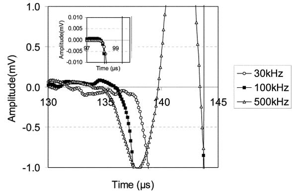
Fig. 7—First arrival according to excitation frequency. In inset figure, onset of excitation pulse.
