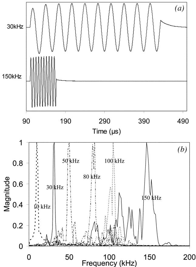
Fig. 5—(a) Examples of electric excitation signals; and (b) Fast Fourier Transform of different tone burst after propagation through mortar.
