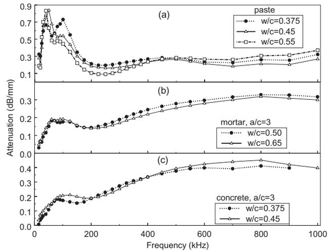
Fig. 3. Effect of  $w/c$  on attenuation variation with respect to frequency of (a) paste (b) mortar with  $a/c = 3$ , (c) concrete with  $a/c = 3$ .
