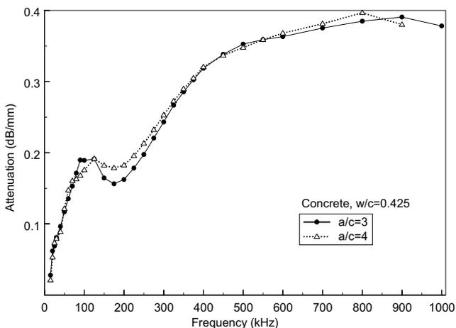
Fig. 5. Effect of  $a/c$  on attenuation variation with respect to frequency of concrete with  $w/c = 0.425$ .
