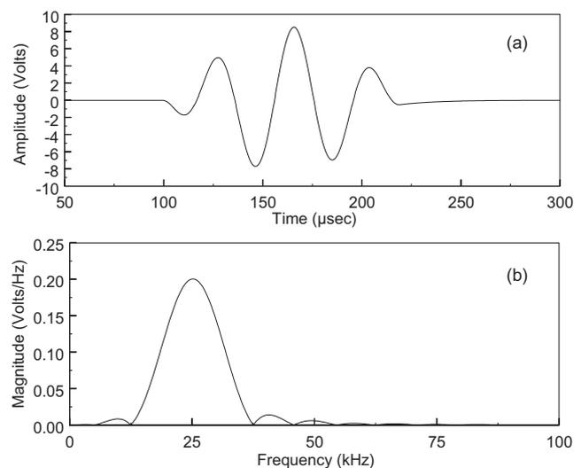
Fig. 1. Input electric signal of 3 cycles at 25 kHz in sinusoidal envelope, (a) in time domain and (b) in frequency domain.
