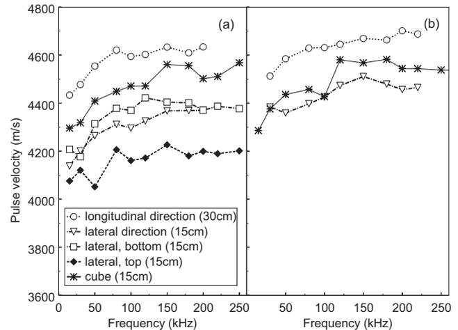
Fig. 7. Effect of specimen geometry on pulse velocity vs. frequency curve obtained using (a) resonant and (b) broadband sensor.
