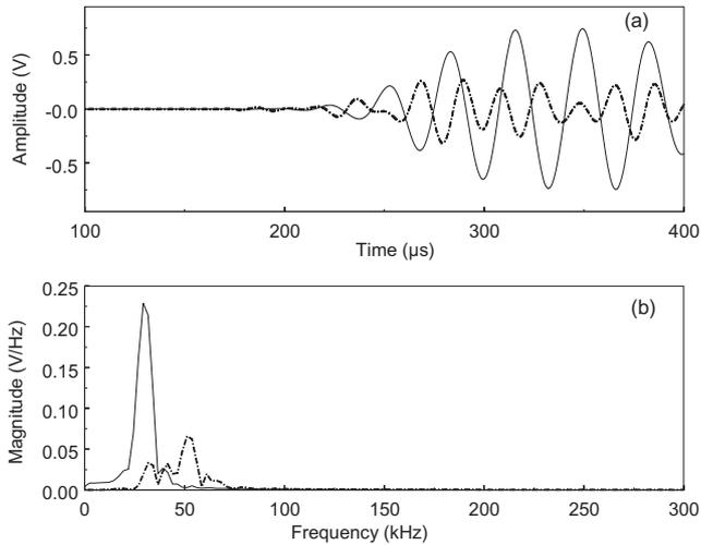
Fig. 8. Tone bursts of 30 (solid) and 50 kHz (dash-dot) after propagation through the cylinder longitudinal direction in (a) time and (b) frequency domain.
