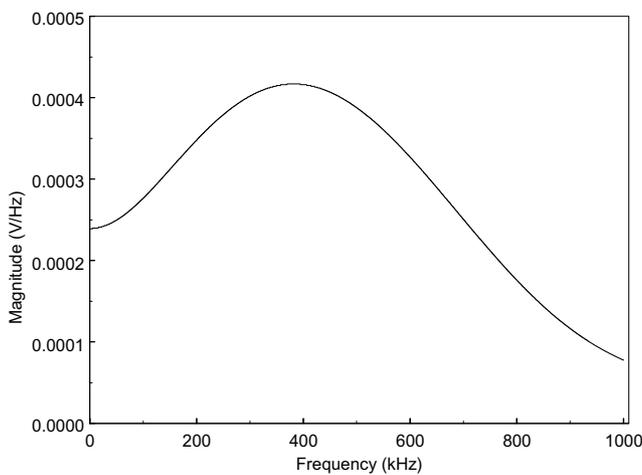
Fig. 15. FFT of 1 cycle of 450 kHz, used for phase velocity calculation.
