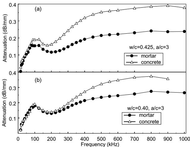
Fig. 2. Effect of aggregate size on attenuation variation with respect to frequency of material with (a)  $w/c = 0.425$  and (b)  $w/c = 0.40$ .
