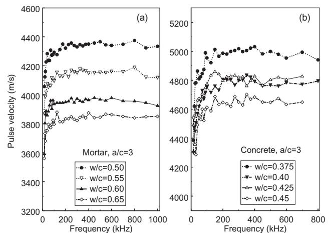
Fig. 12. Effect of  $w/c$  on pulse velocity of (a) mortar and (b) concrete.
