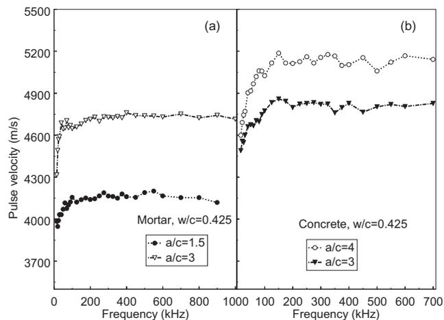
Fig. 13. Effect of  $a/c$  on pulse velocity of (a) mortar and (b) concrete.
