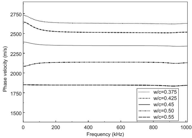
Fig. 18. Effect of  $w/c$  on phase velocity of paste.
