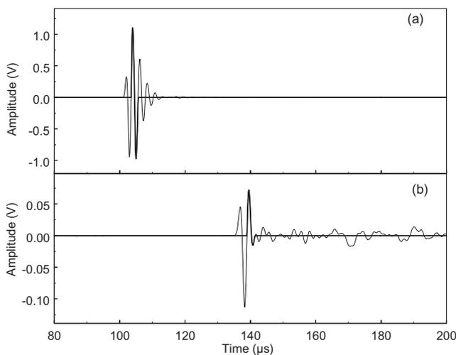
Fig. 16. (a) Sensor face to face and (b) concrete specimen response on the excitation of 1 cycle of 450 kHz. Bold line stands for the part of the signals selected for phase velocity measurements.
