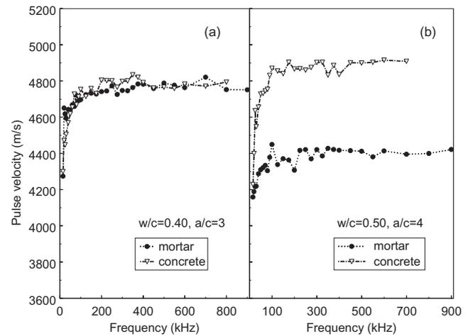
Fig. 14. Effect of aggregate size on pulse velocity of material with (a)  $w/c = 0.40$  and  $a/c = 3$  and (b)  $w/c = 0.50$  and  $a/c = 4$ .
