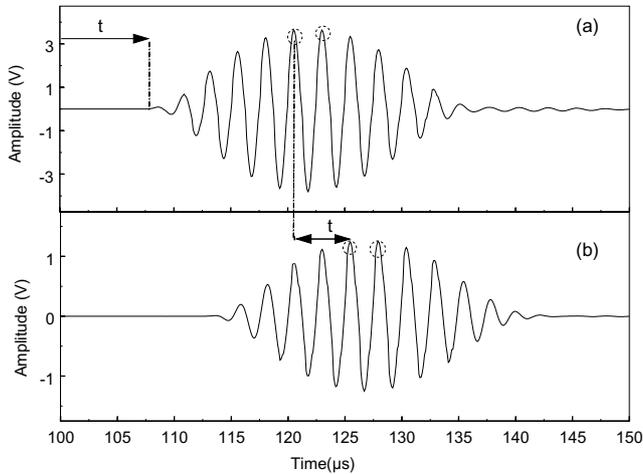
Fig. 6. Tone bursts collected after propagation through different wavepaths in the material.
