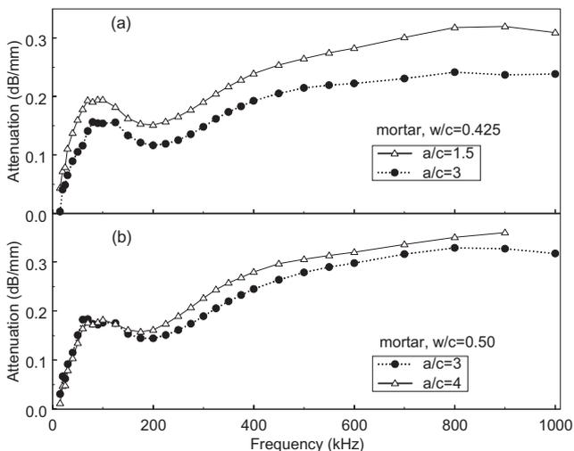
Fig. 4. Effect of  $a/c$  on attenuation variation with respect to frequency of mortar with (a)  $w/c = 0.425$  and (b)  $w/c = 0.50$ .
