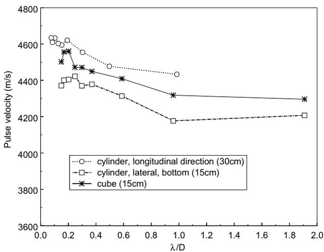
Fig. 9. Effect of specimen geometry on concrete pulse velocity dispersion curves.
