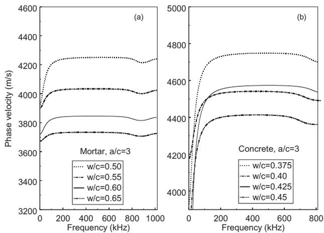
Fig. 19. Effect of  $w/c$  on phase velocity of (a) mortar and (b) concrete.
