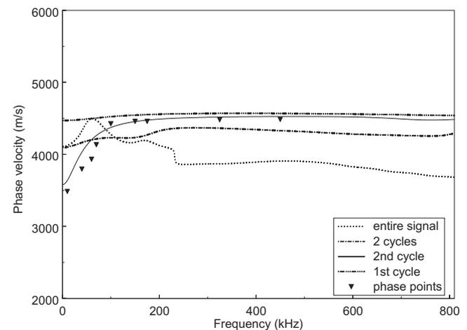
Fig. 17. Concrete phase velocity calculated using different parts of the signal.
