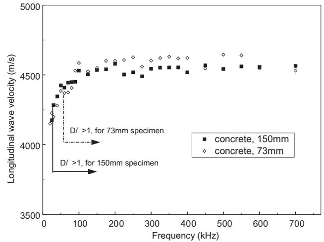
Fig. 10. Effect of specimen size on pulse velocity of concrete.
