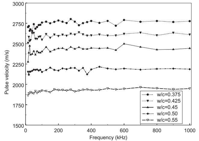
Fig. 11. Effect of  $w/c$  on pulse velocity curves of paste.
