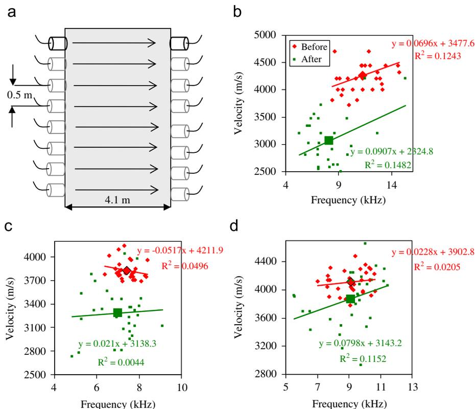
Fig. 1. (a) Schematic representation of the wave measurements, (b)–(d) Correlation plots of pulse velocity vs. central frequency for three different cross sections. Large symbols stand for the average of the populations.
