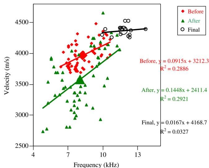
Fig. 2. Correlation plot of pulse velocity vs. central frequency for a cross section of a concrete pier for different times relative to repair. Large symbols stand for the average of the populations.
