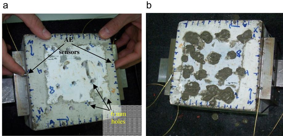
Fig. 3. Measurement of pulse velocity on a concrete cube (a) with drilled holes and (b) the holes were filled with fresh paste.
