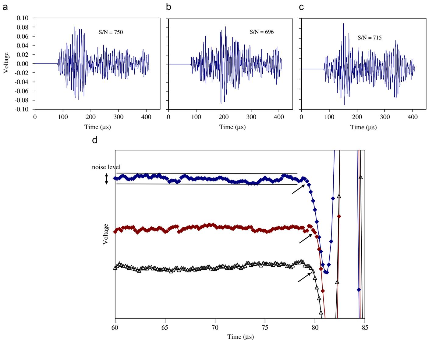
Fig. 4. (a)–(c) Typical received waveforms with their signal-to-noise ratio and (d) zoom at the onset of the waveforms.
