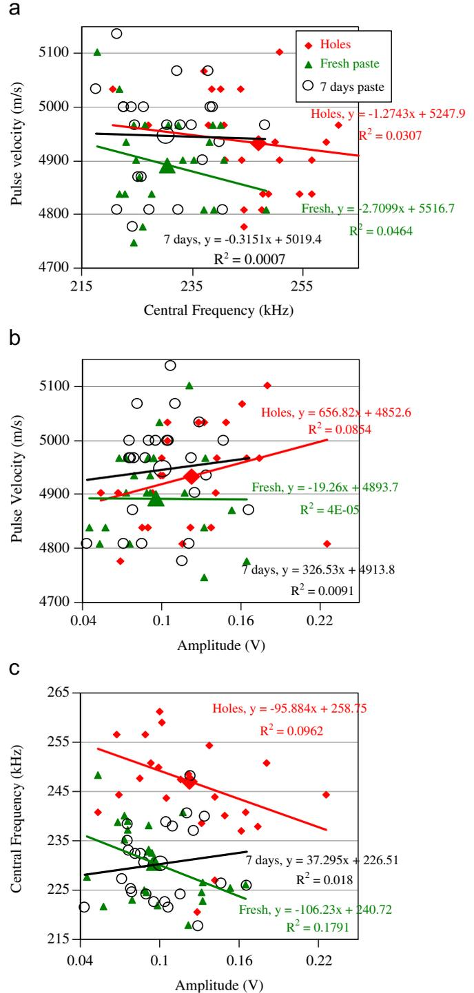
Fig. 5. Correlation plots of (a) pulse velocity vs. central frequency, (b) pulse velocity vs. wave amplitude and (c) central frequency vs. amplitude for the laboratory specimen at three times relative to the application of cement.
