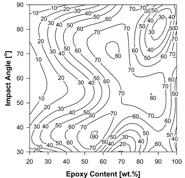
Fig. 3. Contour plot of erosive wear rate of EP-PUR predicted by ANN as a function of epoxy weight content and impact angle of solid particle. Eroder: glass beads, size: 150–300  $\mu\text{m}$ .
