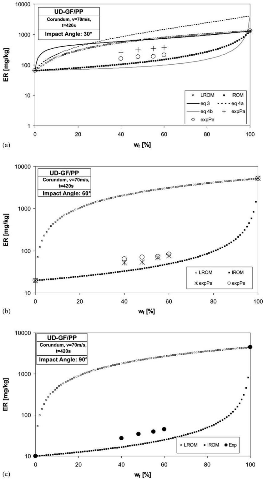
Fig. 5. Application of 'averaging laws of mixture' for the description of the erosion rate (ER) of a composite as a function of the fibre content in the case of a UD-GF/PP composite: (a)  $30^\circ$  impact angle; (b)  $60^\circ$  impact angle and (c)  $90^\circ$  impact angle.
