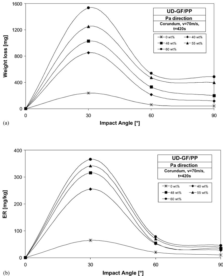
Fig. 1. Weight loss (a) and erosion rate (ER) (b) as a function of impact angle and fibre content of UD-GF/PP composites containing fibres aligned parallel (Pa) to the erosion direction, respectively.
