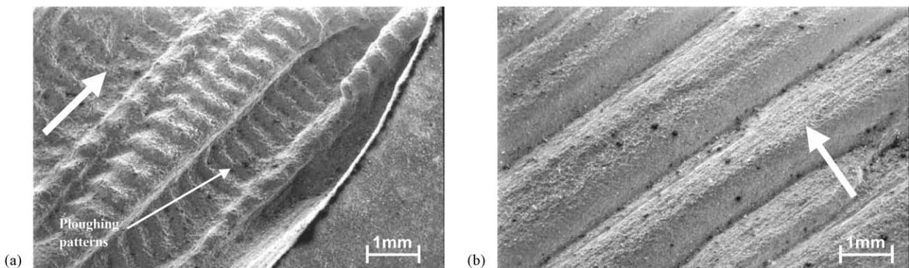
Fig. 4. Scanning electron micrographs taken on the eroded surfaces of GF/PP composites with 40 wt.% fibre content (erosion at  $30^\circ$  angle for 600 s)—illustration of orientation influence on surface topography: (a) parallel (Pa) erosion direction and (b) perpendicular (Pe) erosion direction.
