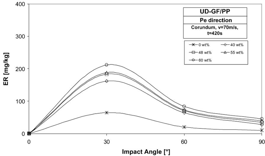
Fig. 2. Erosion rate (ER) as a function of impact angle and fibre content of UD-GF/PP composites containing fibres aligned perpendicular (Pe) to the erosion direction.
