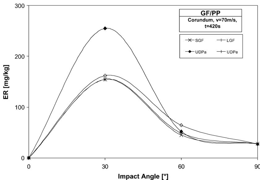
Fig. 3. Erosion rate (ER) as a function of fibre length and fibre-orientation of GF/PP composites at 40 wt.% GF content.
