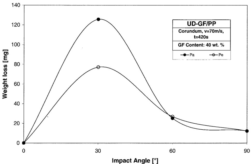
**Figure 2.** Weight loss variation as a function of impact angle and fibre orientation of UD-GF/PP composites. Note: experimental data present the mean value of 3 erosion tests.
