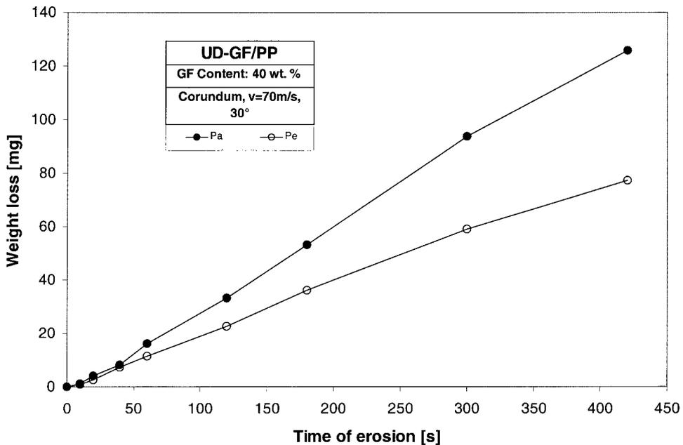
**Figure 3.** Weight loss variation as a function of impact time and fibre orientation of UD-GF/PP composites eroded at 30° impact angle. For note cf. Figure 2.
