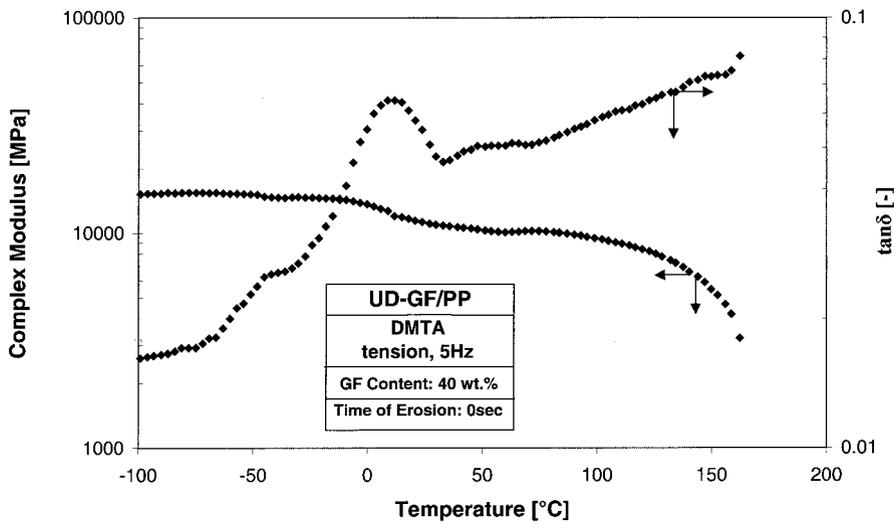
Figure 4. DMTA spectra of the UD-GF/PP before erosion.
