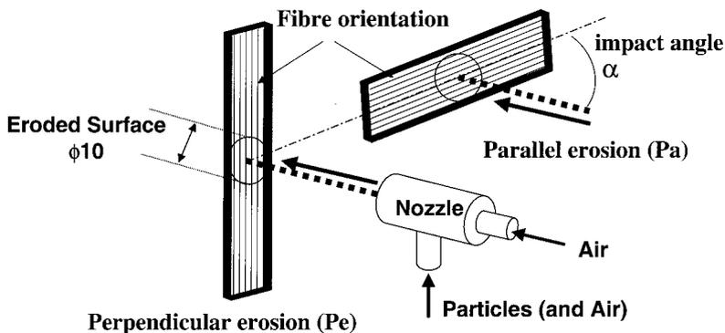
**Figure 1.** Schematic representation of the erosion test set-up. Note: this figure indicates the erosion direction and the related designation of the UD composites.
