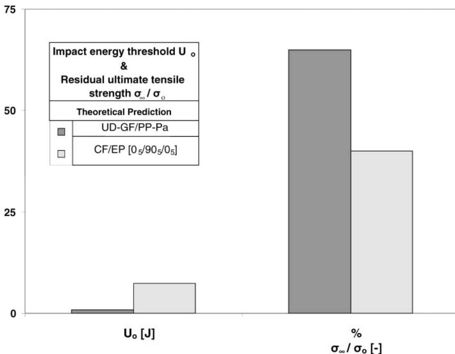
**Figure 6.** Comparison of the impact energy threshold ( $U_o$ ) and the normalised ultimate residual tensile strength ( $\sigma_\infty/\sigma_o$ ) after solid particle erosion of GF/PP ( $v_f=20\%$ ) and CF/EP ( $v_f=60\%$ ) systems
