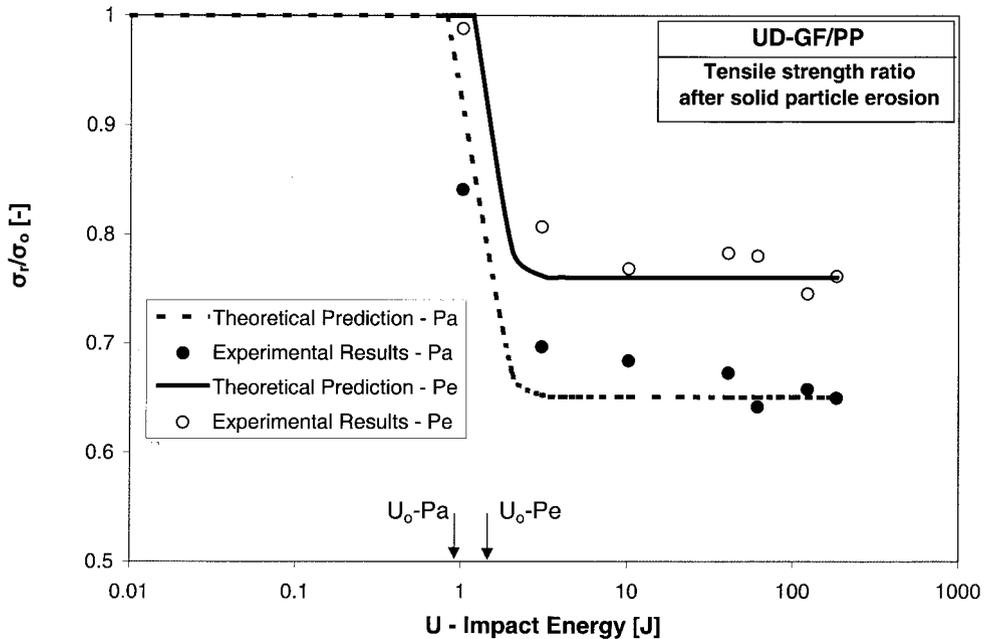
**Figure 5.** Experimental values and theoretical prediction of the normalised residual tensile strength, ( $\sigma_r/\sigma_o$ ) of UD-GF/PP due to solid particle Pa- and Pe-erosion as a function of the impact energy ( $U$ ).
