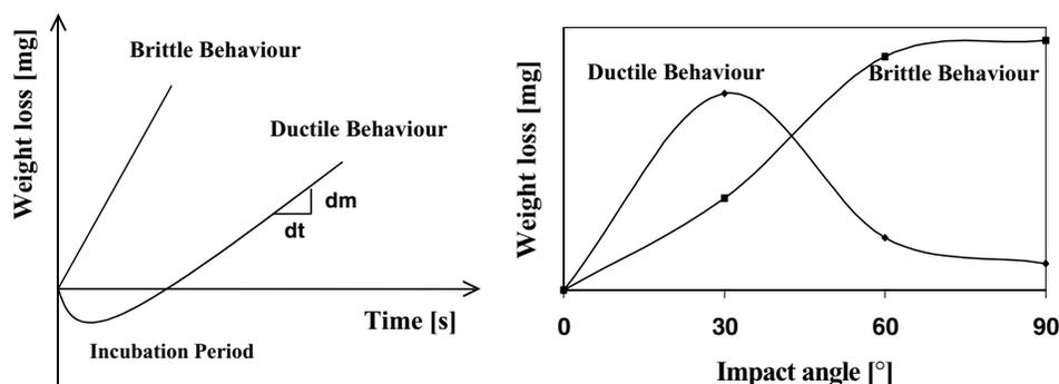
Figure 1 Typical behaviours in erosion schematically.
