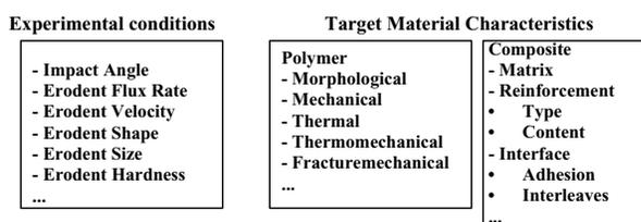
Figure 3 Parameters influencing the solid particle erosion.
