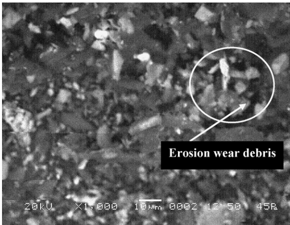
Fig. 2. SEM image of the eroded surface of glass-polyester SiC hybrid composite showing fiber and matrix micro-flake debris.
