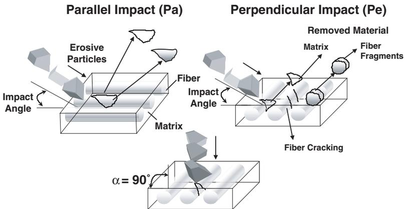
**Figure 5.** Scheme of the role of the interface on the erosion of UD fiber-reinforced composites under parallel (Pa) and perpendicular (Pe) impact conditions.
