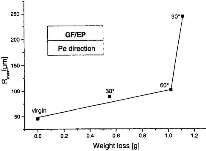
Figure 7. Change of the roughness parameter  $R_{max}$  as a function of impact angle for GF/EP-M tested in Pe direction.
