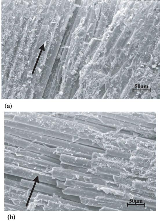
**Figure 4.** SEM micrographs taken on the eroded surface of composites impacted at 30° angle for 40s Designation: (a) GF/EP-Pa and (b) GF/EP-Pe.
