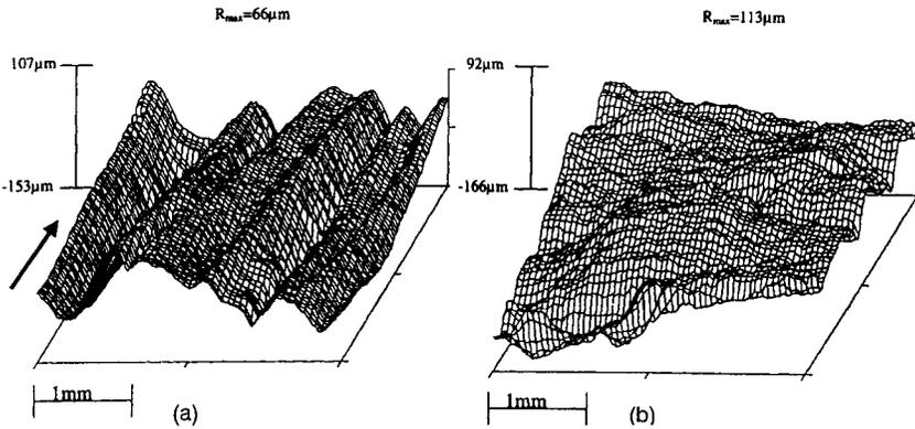
Figure 8. 3D roughness contour of GF/EP composite eroded in Pa direction for 40s Designation: (a) 30° and (b) 90°. Note: this figure shows that brittle erosion occurred and that  $R_{max}$  changes parallel with the erosion rate.
