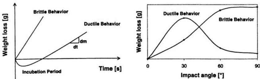
Figure 2. Schematic diagram of brittle and ductile type erosive wear.
