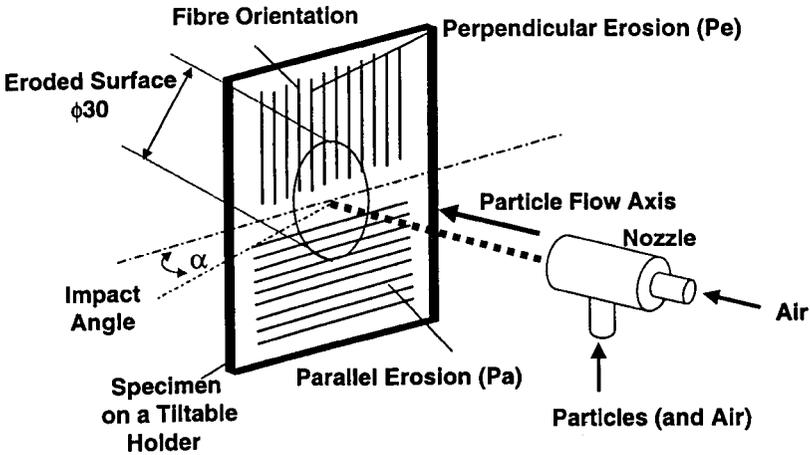
**Figure 1.** Test set-up to study the solid particle erosion of UD fiber reinforced composites schematically.
