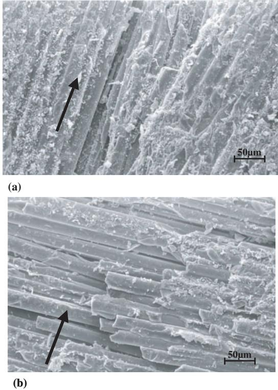
**Figure 4.** SEM micrographs taken on the eroded surface of composites impacted at  $30^\circ$  angle for 40s Designation: (a) GF/EP-Pa and (b) GF/EP-Pe.
