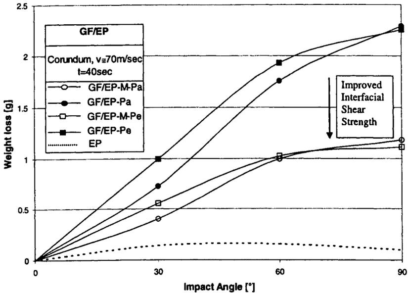
**Figure 3.** Influence of impact angle, erosion direction and interface modification on the erosive wear of EP and GF/EP composites.
