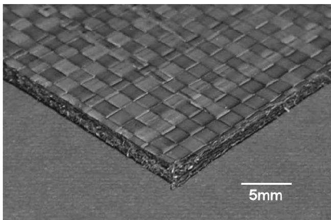
Fig. 4. Photograph of an all-PP composite laminate, in which the plain weave of the fabric is clearly visible on the upper surface of the laminate. Although manufactured from woven highly oriented PP tapes, these tapes are easily fibrillated, and the fibrillar nature of the tapes is clearly visible on the edge of the laminate.
