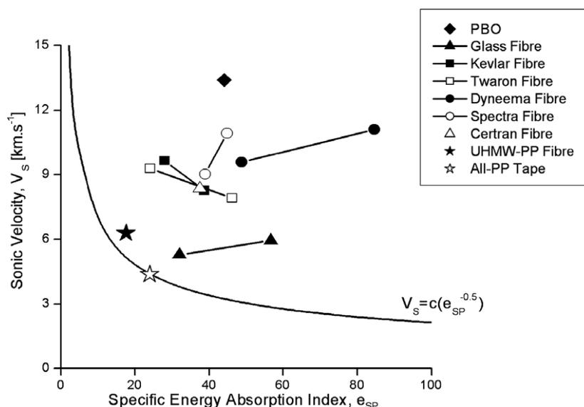
Fig. 1. Specific energy absorption capability index vs. sonic velocity for various fibres showing the curve predicting equal ballistic energy absorption performance based on Eq. (6). Data taken from Table 1.
