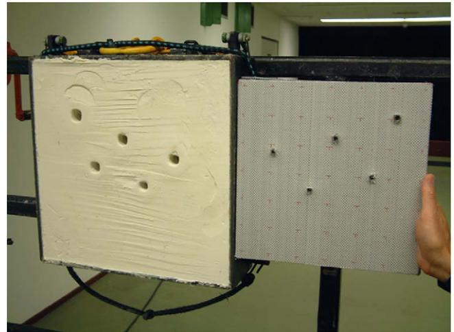
Fig. 7. Ballistic impacted all-PP plate (right) with plasticine backing (left) showing five clear perforations.
