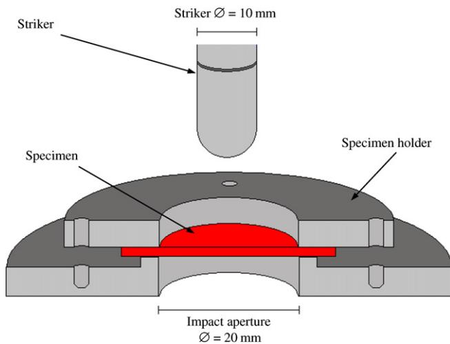
Fig. 5. Schematic of falling weight impact test set-up showing impact striker, specimen and specimen holder.
