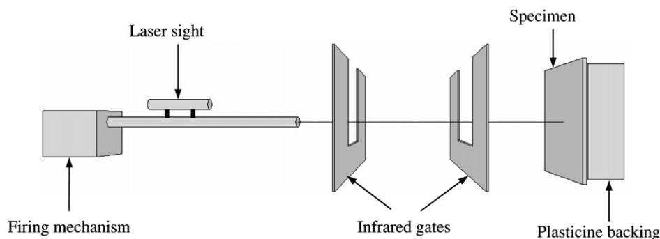
Fig. 6. Schematic of ballistic impact test set-up consisting of firing mechanism, infra-red velocity gates and impact specimen with plasticine backing (not to scale). The total distance from firing mechanism to specimen is  $10\text{ m}$ .
