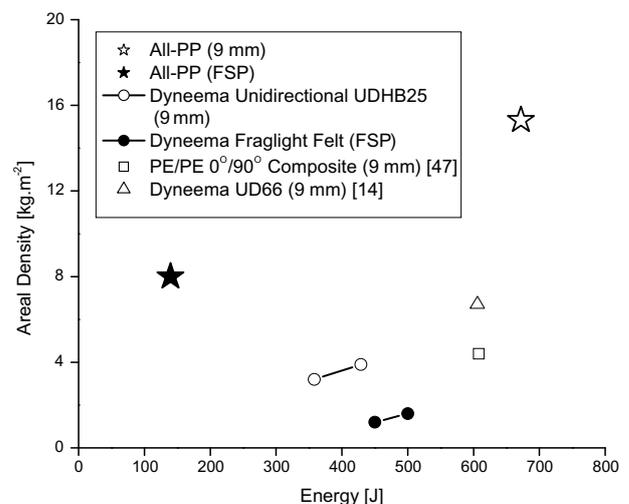
Fig. 11. Comparison of different polyolefin structures for ballistic impact resistance showing that all-PP composite laminates require a much greater areal density to absorb the energy of ballistic impacts when compared to polyethylene alternatives.
