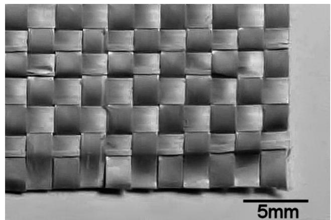
Fig. 3. Photograph of the woven all-PP tape fabric, prior to consolidation into composite laminates.
