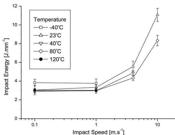
Fig. 8. Falling weight penetrative impact energy vs. impact speed for a range of impact temperatures showing the effect of increasing impact velocity and impact temperature.
