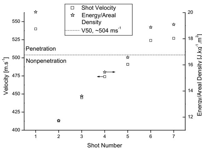
Fig. 10. Ballistic V50 determination of an all-PP composite plate giving a V50 value (the velocity at which, statistically, the probability of perforation is 50%) of  $504 \text{ m s}^{-1}$ . It must be stated that this V50 value is specific to the particular plate and projectile being investigated, in this case a  $1.1 \text{ g}$  FSP.
