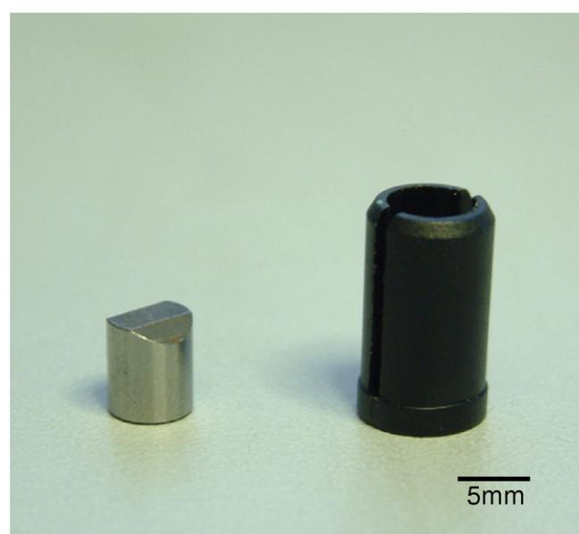
Fig. 2. Fragment simulating projectile (FSP) (left) with plastic sabot (right) for ballistic testing designed to simulate impact by explosion fragments. The FSP has a diameter of 5.39 mm and length of 6.35 mm.
