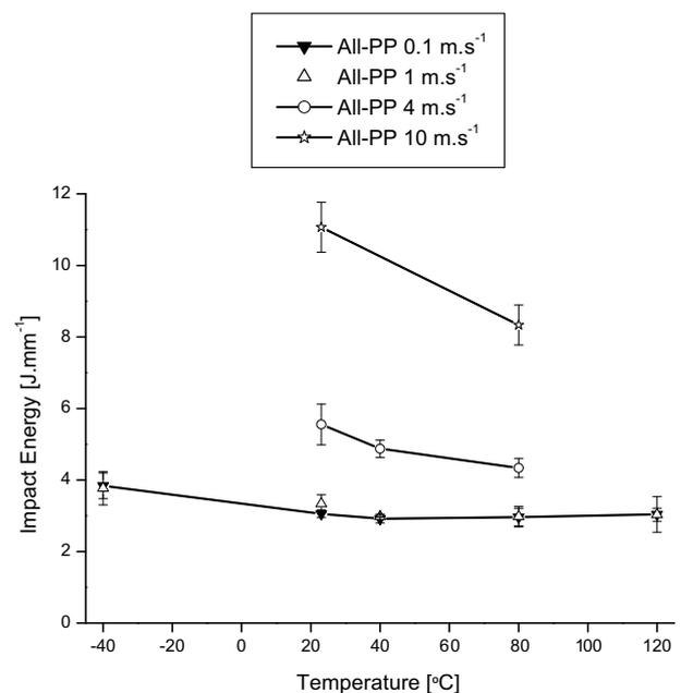
Fig. 9. Falling weight penetrative impact energy vs. impact temperatures for a range of impact speeds and temperatures, further illustrating the relatively large effect of impact velocity but rather small effect of impact temperature.
