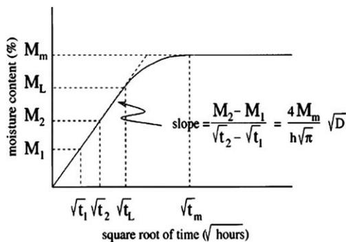
Fig. 1. Illustration of the change of moisture content with the square root of time for Fickian diffusion. For  $t < t_L$  the slope is constant [48].
