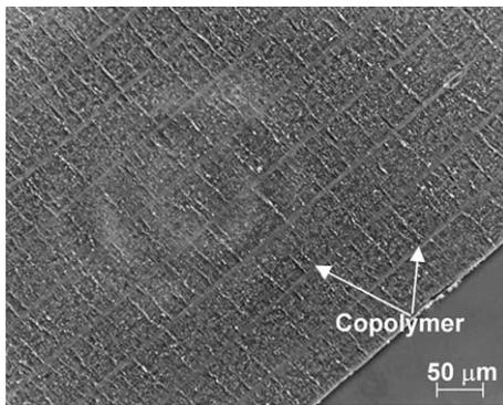
Fig. 3. Optical micrograph under transmitted light of the microtomed cross-section of a compacted unidirectional specimen [50].
