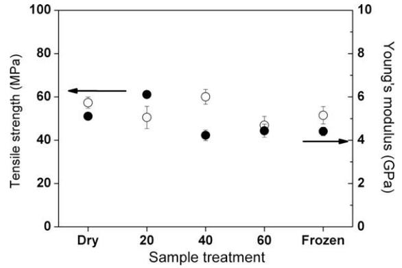
Fig. 13. Mechanical properties of GMT composites before (dry) and after nearly 40 days immersion in water at different temperature (20 °C, 40 °C and 65 °C) and subsequently freezing.
