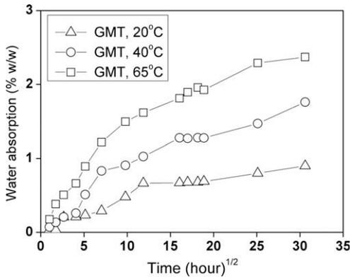
Fig. 10. Water absorption curve for GMT specimen as a function of square root of time.
