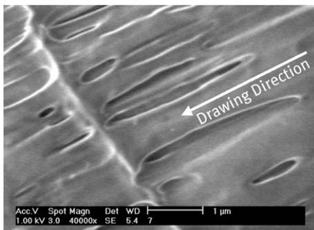
Fig. 4. ESEM of drawn all-PP tape after permanganate etching showing intra-tape voids [42].
