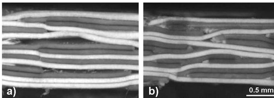
Fig. 2. (a) All-PP woven fabric composite compacted at 0.1 MPa pressure at 145 °C and (b) 4 MPa pressure at 145 °C. Inter-tape voids can still be seen between adjacent tapes in the crimp region even at high pressure consolidation [27].
