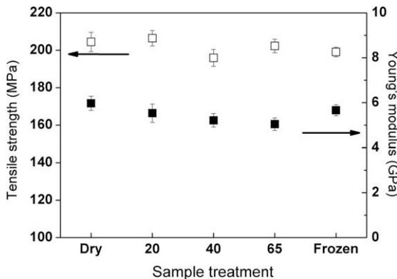
Fig. 12. Mechanical properties of all-PP composites before (dry) and after nearly 40 days immersion in water at different temperature (20 °C, 40 °C and 65 °C) and subsequently freezing.
