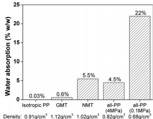
Fig. 5. Weight fraction of water absorbed by various polypropylene composites after 1-month immersion in distilled water. All-PP composites are suffixed by the pressure used to consolidate the laminates (4 MPa by hot pressing or 0.1 MPa by vacuum bagging routes).
