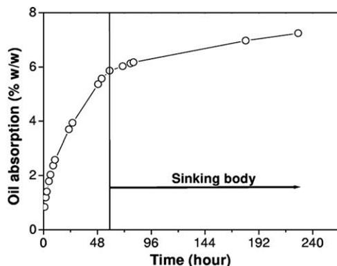
**Fig. 7.** Oil absorption as a function of time. During the third day of immersion in oil, the density of the all-PP specimen is higher than that of the oil and the specimen sinks.
