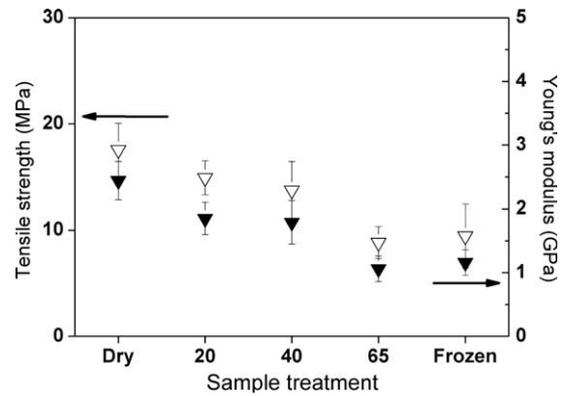
Fig. 14. Mechanical properties of NMT composites before (dry) and after nearly 40 days immersion in water at different temperature (20 °C, 40 °C and 65 °C) and subsequently freezing.
