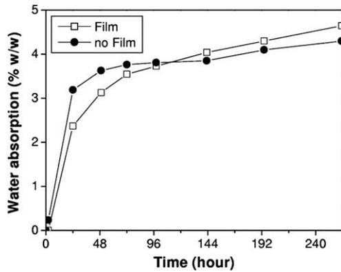
**Fig. 6.** Water absorption as a function of time of all-PP compacted at 145 °C and 4 MPa pressure. The top and bottom faces of one specimen were sealed by 30 μm thick PP films. Note the similarity between the two laminates indicating that water absorption mainly occurs through the edges.
