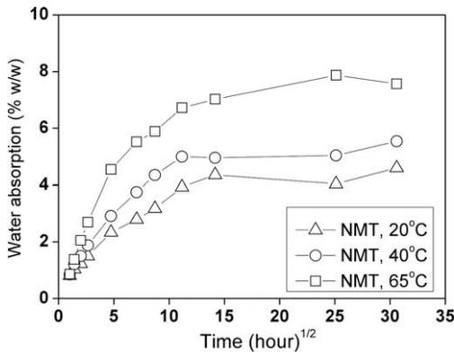
Fig. 11. Water absorption curve for NMT specimen as a function of square root of time.
