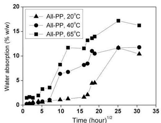
**Fig. 9.** Water absorption curve for all-PP specimen as a function of square root of time.
