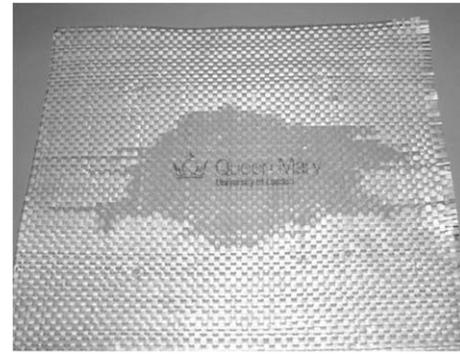
**Fig. 8.** Oil absorption by woven all-PP tapes. The normally opaque tapes become transparent when in contact to a small volume of oil in the centre of the fabric. This change in optical properties is thought to be due to oil filling the voids within the PP tapes, reducing the amount of light scattered by the voids.
