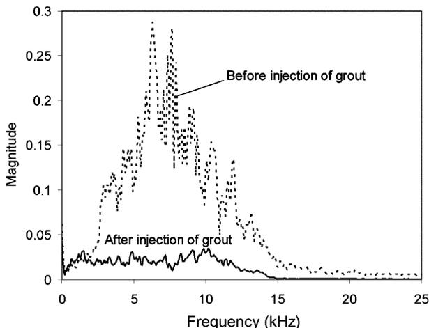
Fig. 5—Typical FFTs of signals recorded at actual structure.
