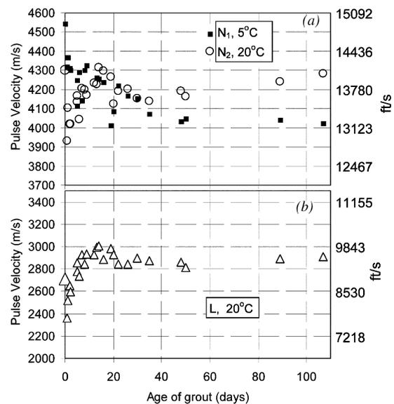
Fig. 3—Pulse velocity of porous concrete specimens before and at different ages after impregnation with grout: (a) normalweight aggregates; and (b) lightweight aggregates. (Note: 1 °C = 33.8 °F.)
