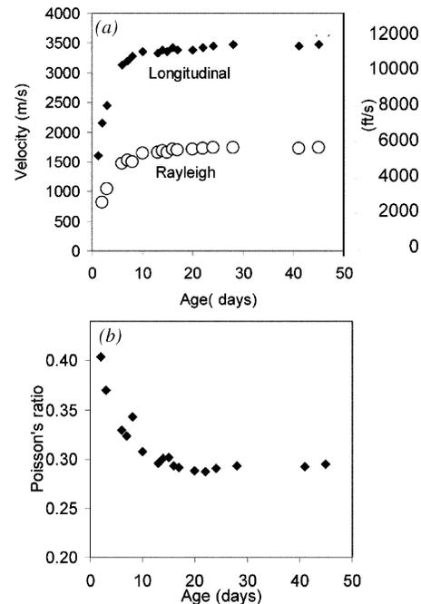
Fig. 2—Development of: (a) wave velocity; and (b) Poisson's ratio of grout with age.
