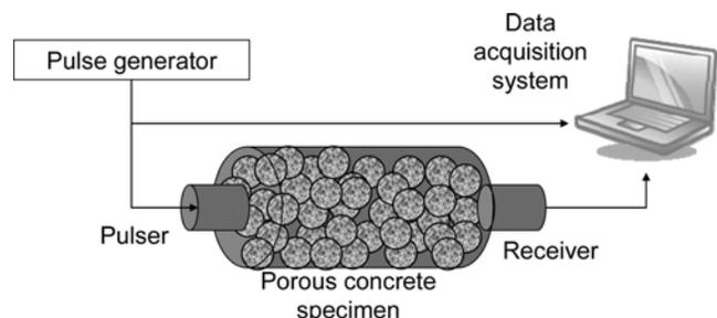
**Fig. 1—Experimental setup for porous concrete pulse velocity measurement.**
