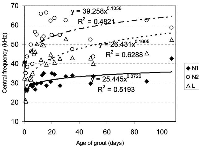
Fig. 4—Central frequency of waveforms of porous concrete specimens before and at different ages after impregnation with grout.
